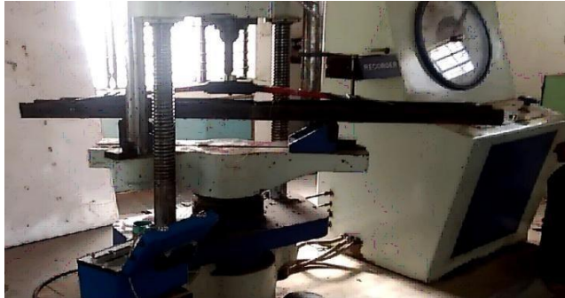
Fig. 3: Experimental Testing on Composite Leaf Spring.
